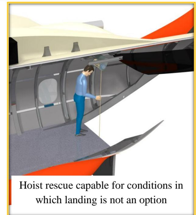
Hoist rescue capable for conditions in which landing is not an option
