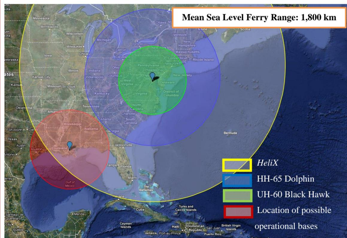
**LEFT:** The red circle seen in the figure to the left has a radius of 600 km centered on New Orleans, LA and the circumference indicates all the possible locations the operational base could be located. If **deployed from the US Coast Guard Surface Forces Logistics center**, in Baltimore, MD, the *HeliX* clearly outperforms both the Dolphin and the Black Hawk, and is the only vehicle capable of reaching base camp without refueling.
