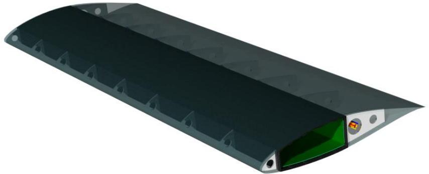
One of the unique selling points of the *HeliX* is its implementation of aerodynamically deployed **outboard wing extensions (OWEs)**.
