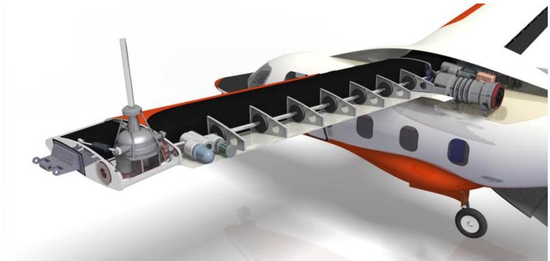
The *HeliX* was designed with *turboshaft engines*, based on the 2007 AHS Student Design Competition “rubber” engine model, for increased reliability and minimized cost.
