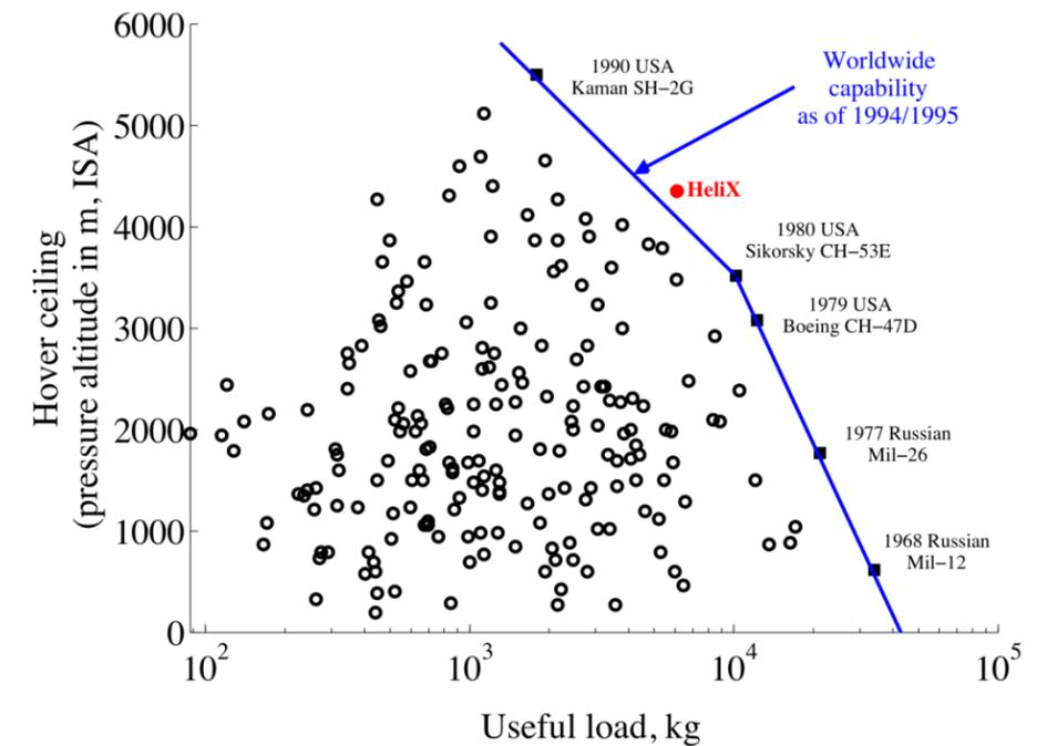
It should be noted that the *HeliX*'s performance characteristics exceed the mission specifications due to the requirement to satisfy a 6 metric ton useful load in each mission set by the RFP. Had the *HeliX* only been sized to perform with the mission specific payloads, the vehicle would have been significantly smaller.
