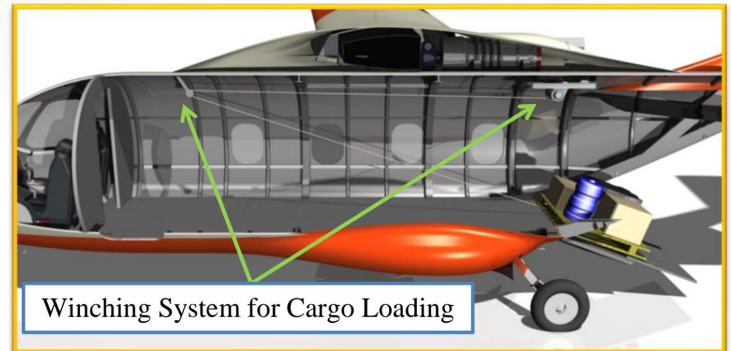
Winching System for Cargo Loading
