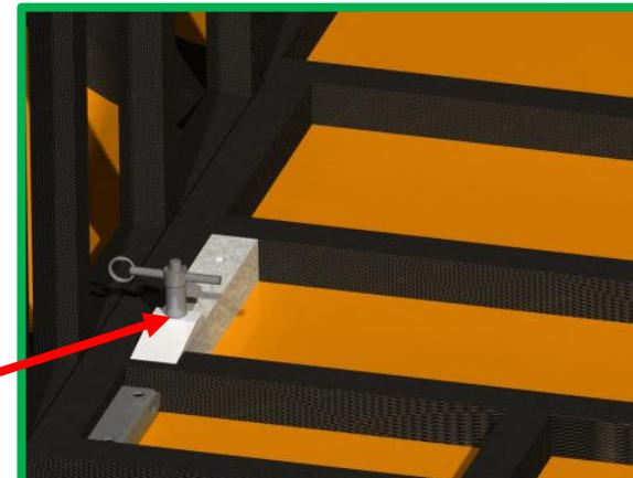
Adjustable stops and fuselage frame position payload
