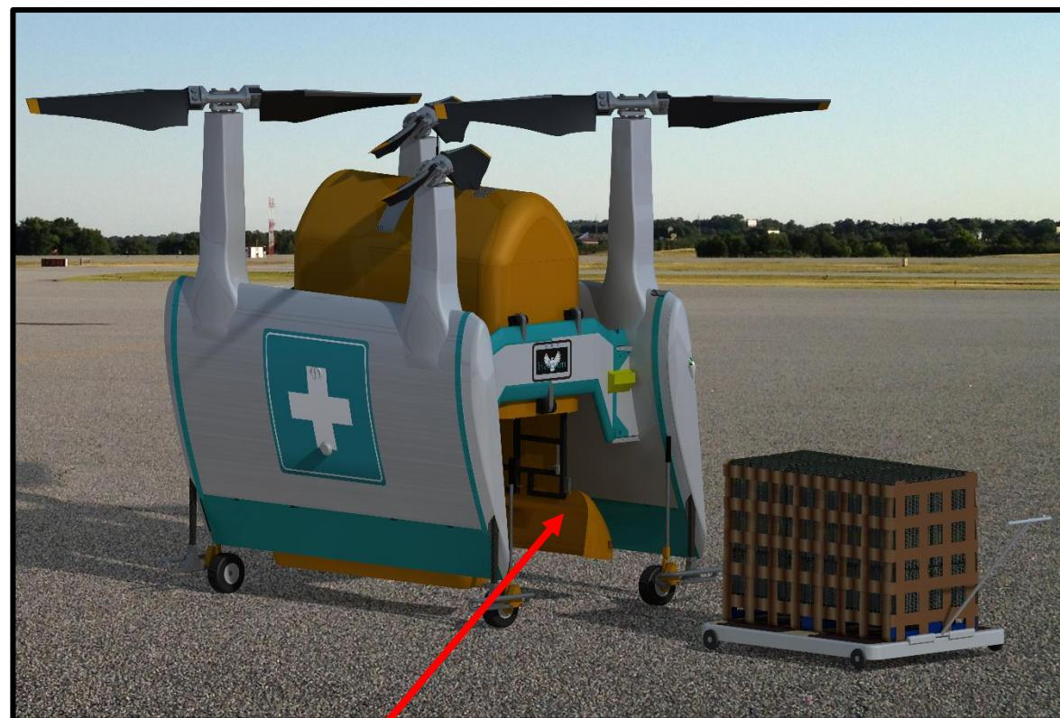
Payload doors operable by hand and latch open
