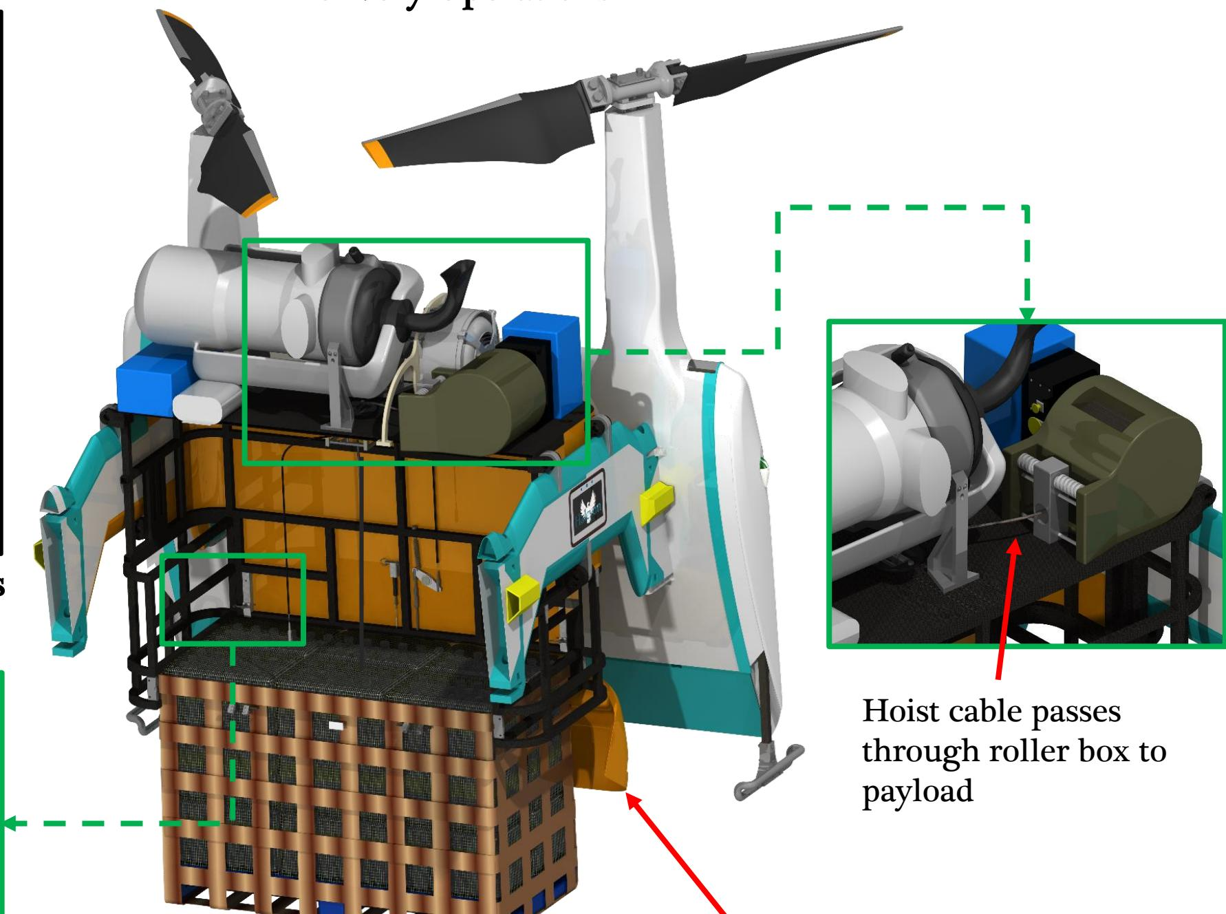
Hoist cable passes through roller box to payload
