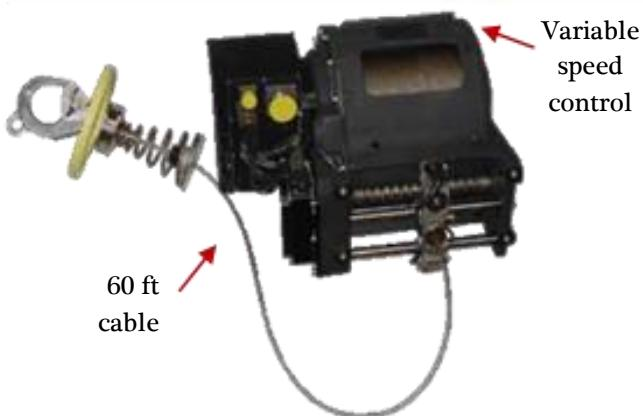
*Halcyon*'s cargo delivery system includes a variable-speed hoist designed for helicopter rescue operations to deliver the payload within 30 seconds, well under the 60 second requirement, and an automatic pressure-sensitive cargo hook to release the payload after impact with complete autonomy.
