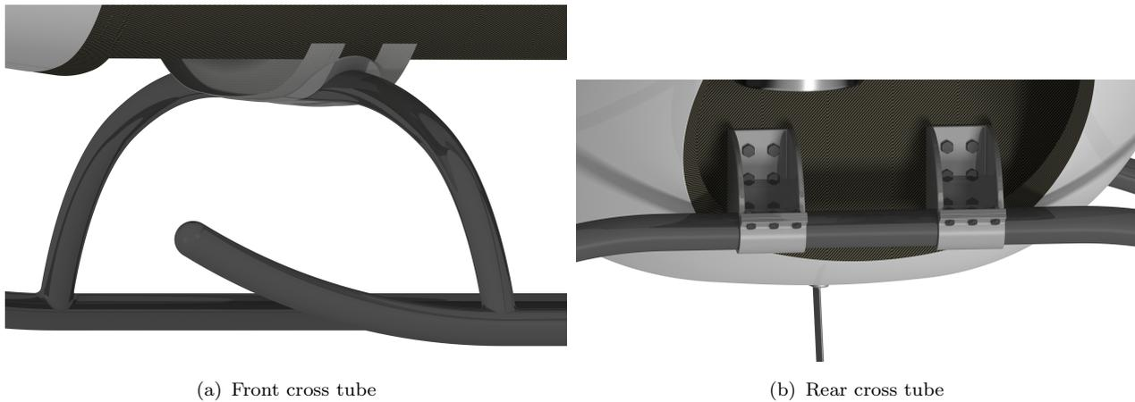
FIGURE 17.1: Mounting position of: (a) Front cross tube between fiberglass bulkheads, and (b) Rear cross tube to aft bulkheads.
