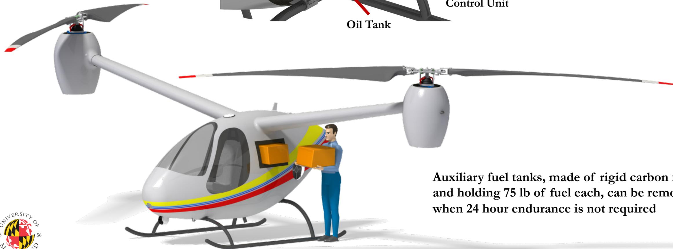
Auxiliary fuel tanks, made of rigid carbon fiber and holding 75 lb of fuel each, can be removed when 24 hour endurance is not required
