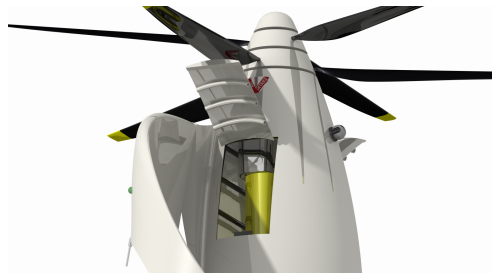
FIGURE 13.1: Door providing access to the engine bay
