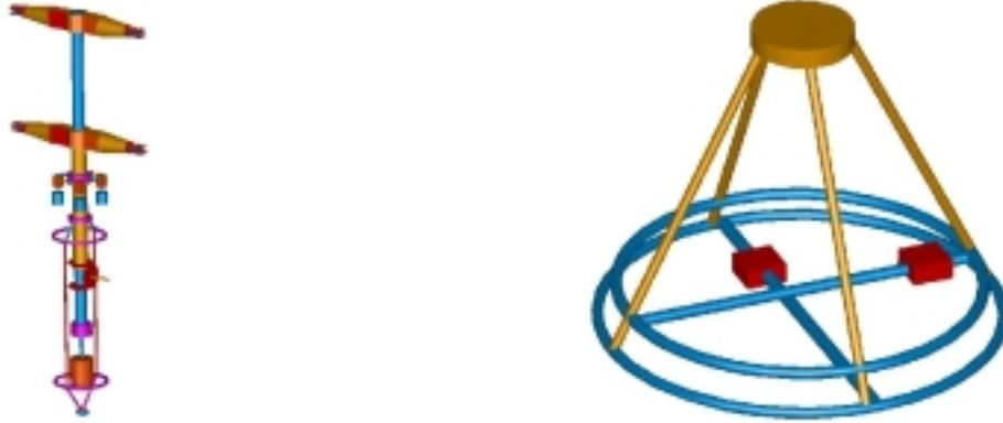
Figure 13.2: Control by shaft tilt and CG shift
