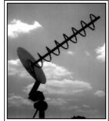
Figure 17.5: Helical antenna
