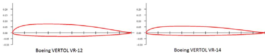
**Figure 2: Cross-Sectional Shapes of Airfoils Used in Design**
