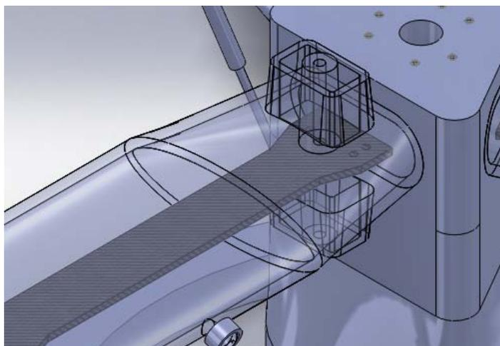
**Figure 5: Close-up of Slot, Cuff, and Elastomeric Cone Coupling on Rotor Blade**
