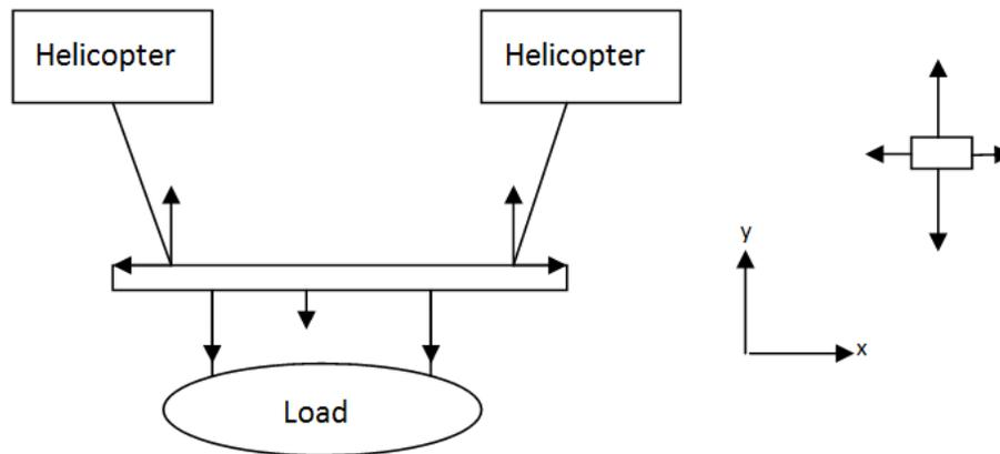
**Figure 12: Connection Schematic and Free-Body Diagram for Direct Connection**
