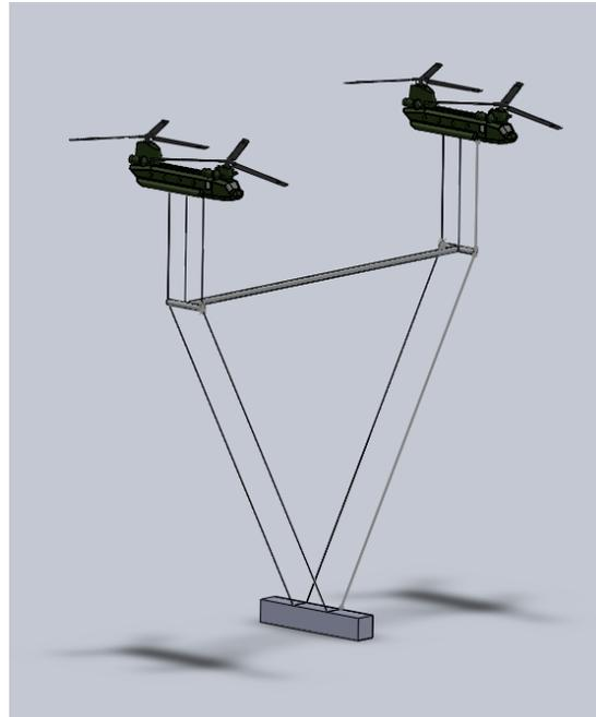
**Figure 16: Flight Configuration**
