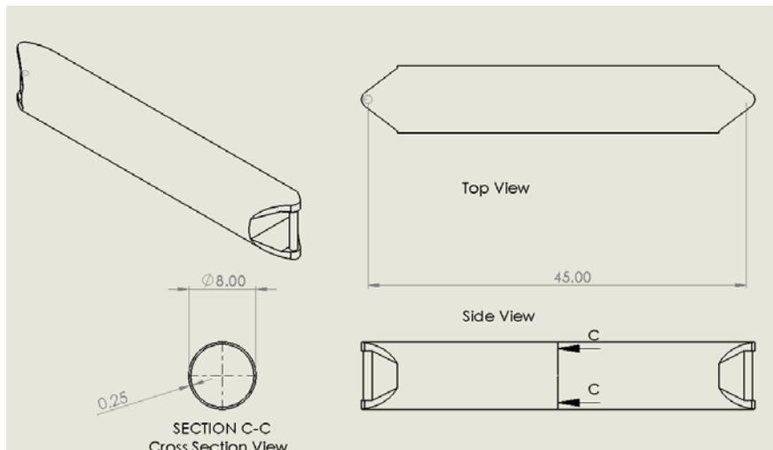
**Figure 8: Single Shaft Section (Units in Inches)**
