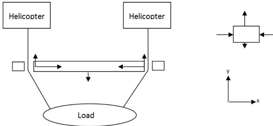
**Figure 13: Connection Schematic and Free-Body Diagram for Cable Stay**
