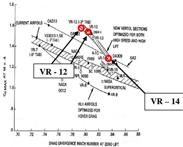
**Figure 1: Rotorcraft Airfoil Performance Comparison**
