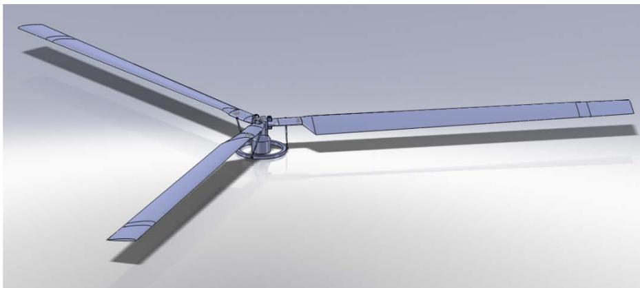
**Figure 4: Assembled Rotor with 3 Blades**
