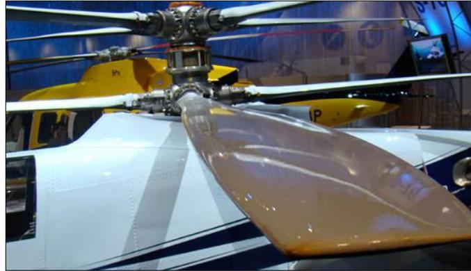
Figure 8 Sikorsky X2 Bearingless Hub
