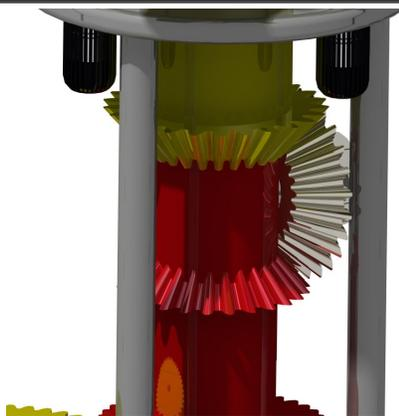
A structural shaft connecting the base of the rotor hub to the nose portion of the hub
