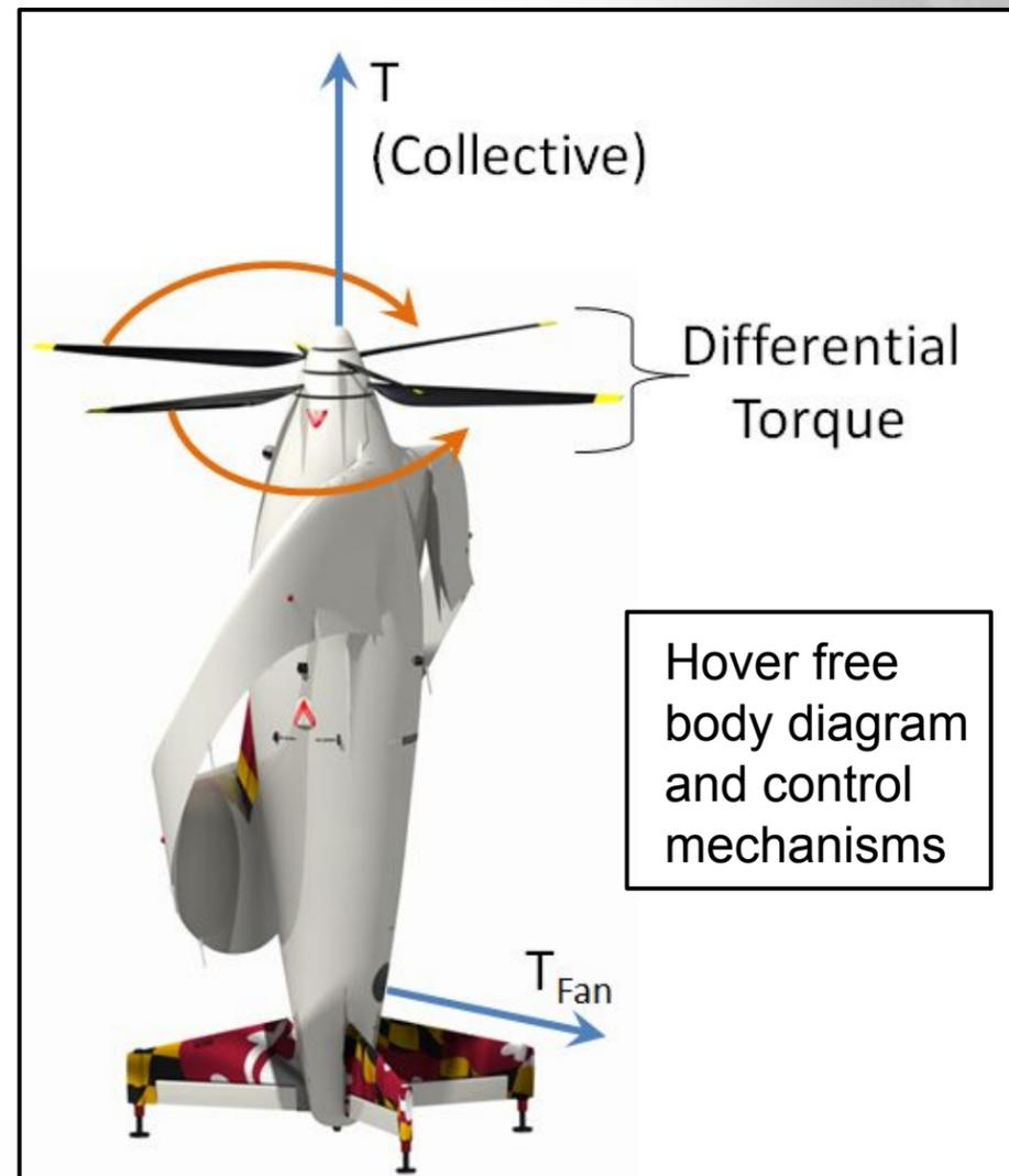
Hover free body diagram and control mechanisms
