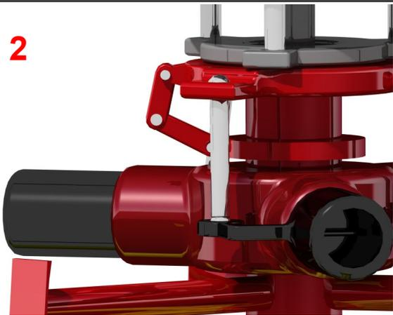
Blade grips take advantage of centrifugal forces to grip composite rotor blades
