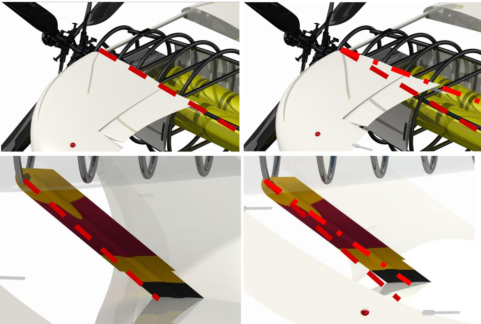
The two images on the left depict the wing and the strut that connects the bottom wing to the fuselage in their static position. The wing is pitched down  $5^\circ$  in the images to the right with the dotted red line depicting the change in wing incidence.
