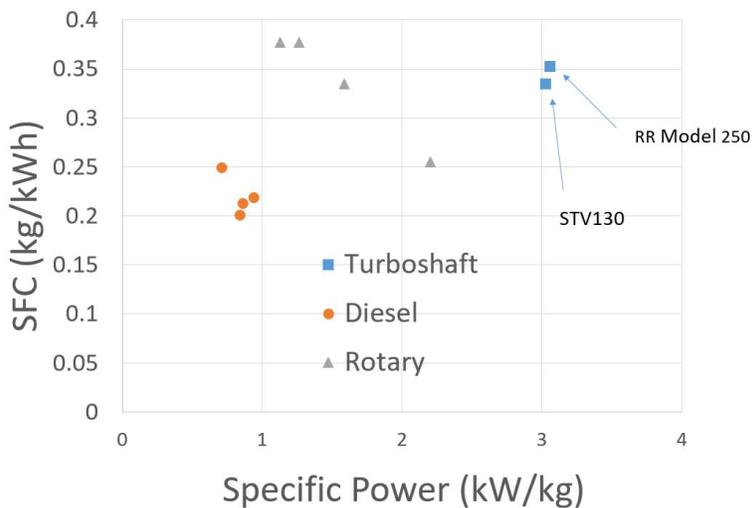
Comparison of Rotary, Diesel, and Turboshaft engines
