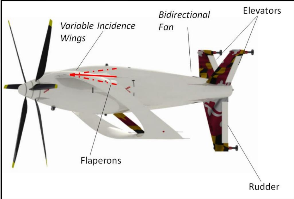
Forward flight control mechanisms
