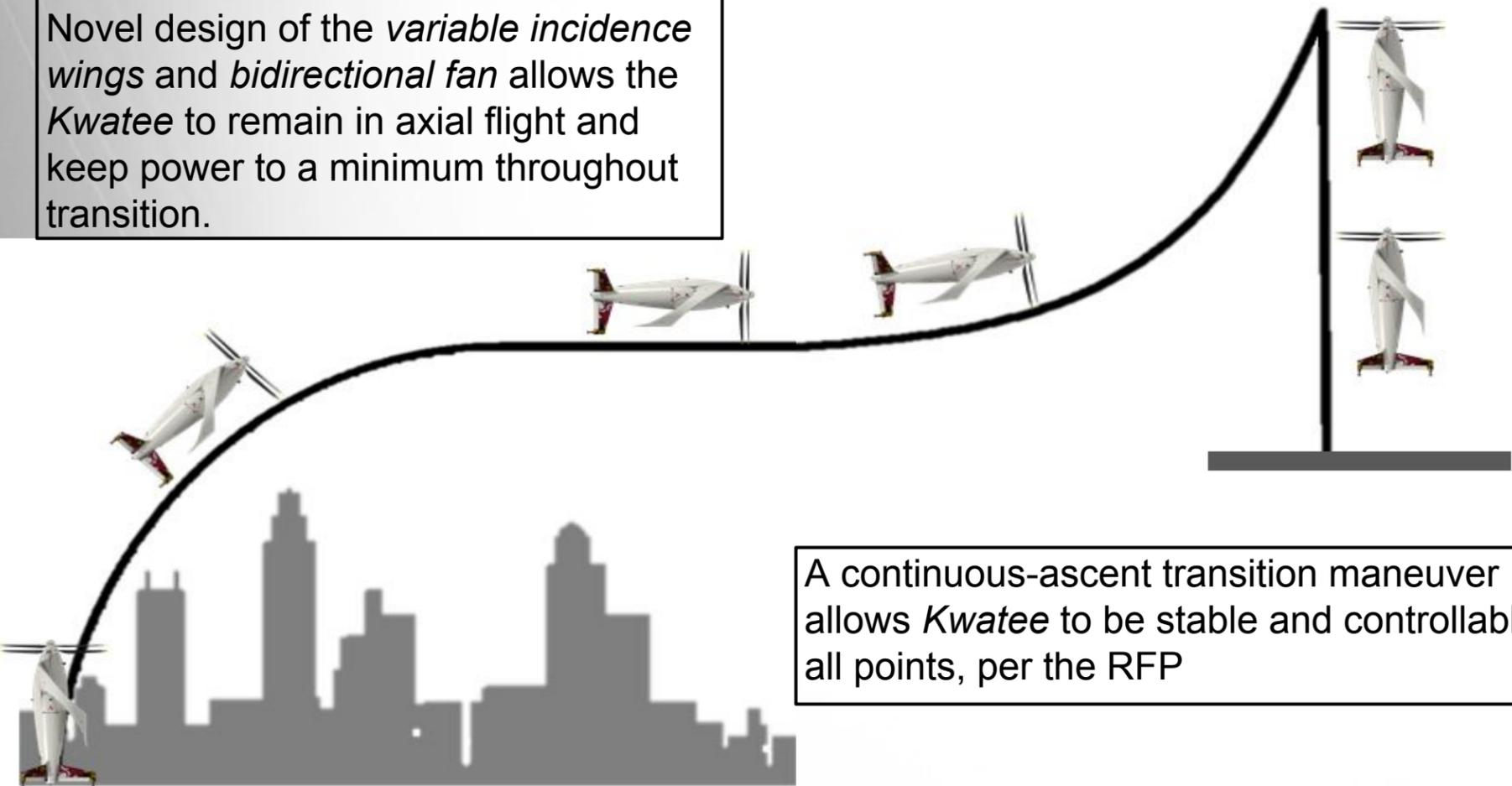
A continuous-ascent transition maneuver allows Kwatee to be stable and controllable at all points, per the RFP
