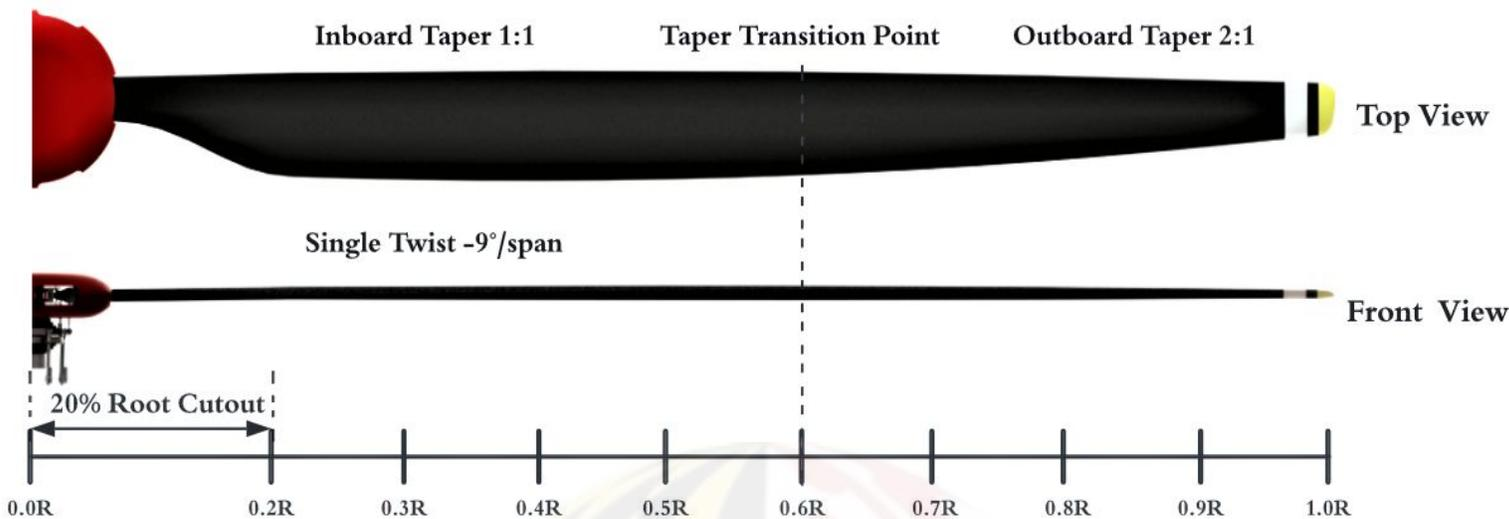
Blitzen's main rotor blades were designed using team-developed BEMT code for optimal hover and cruise performance and minimal noise production.
