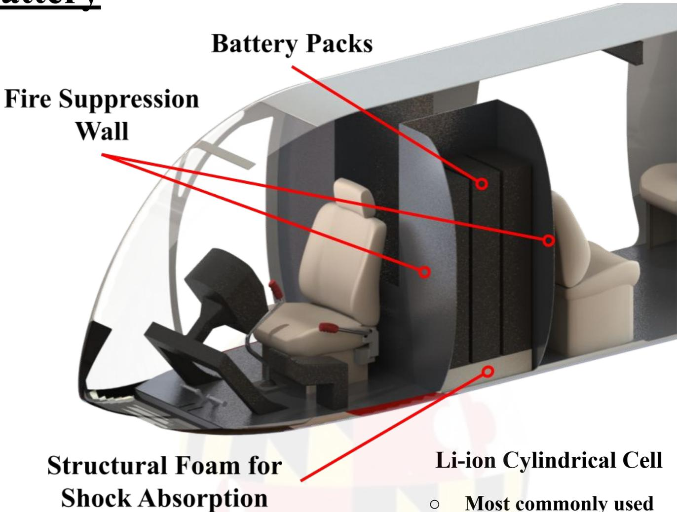
**Structural Foam for Shock Absorption**
