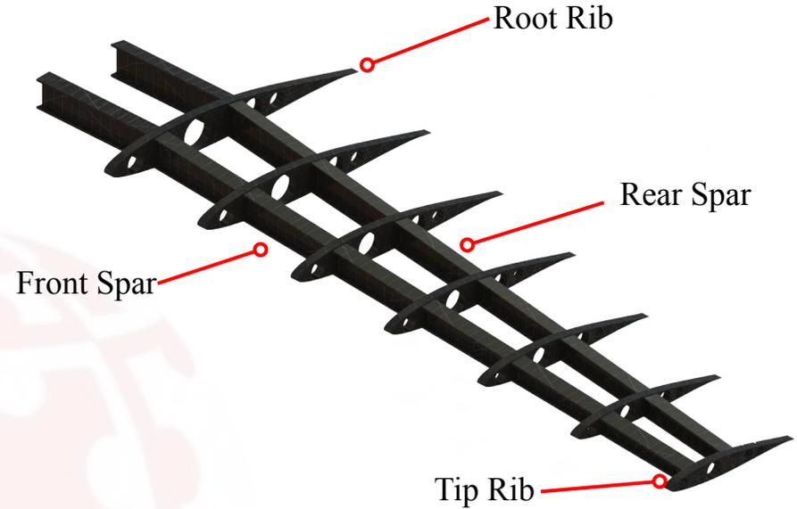
Wing structure with 7 ribs on each wing
