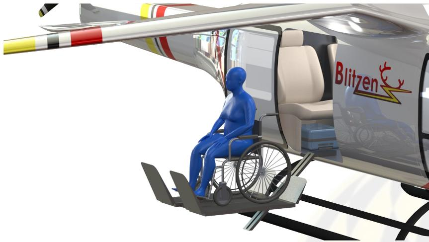
Retractable, motorized ingress/egress lift for passengers with wheelchairs will be stored at landing sites
