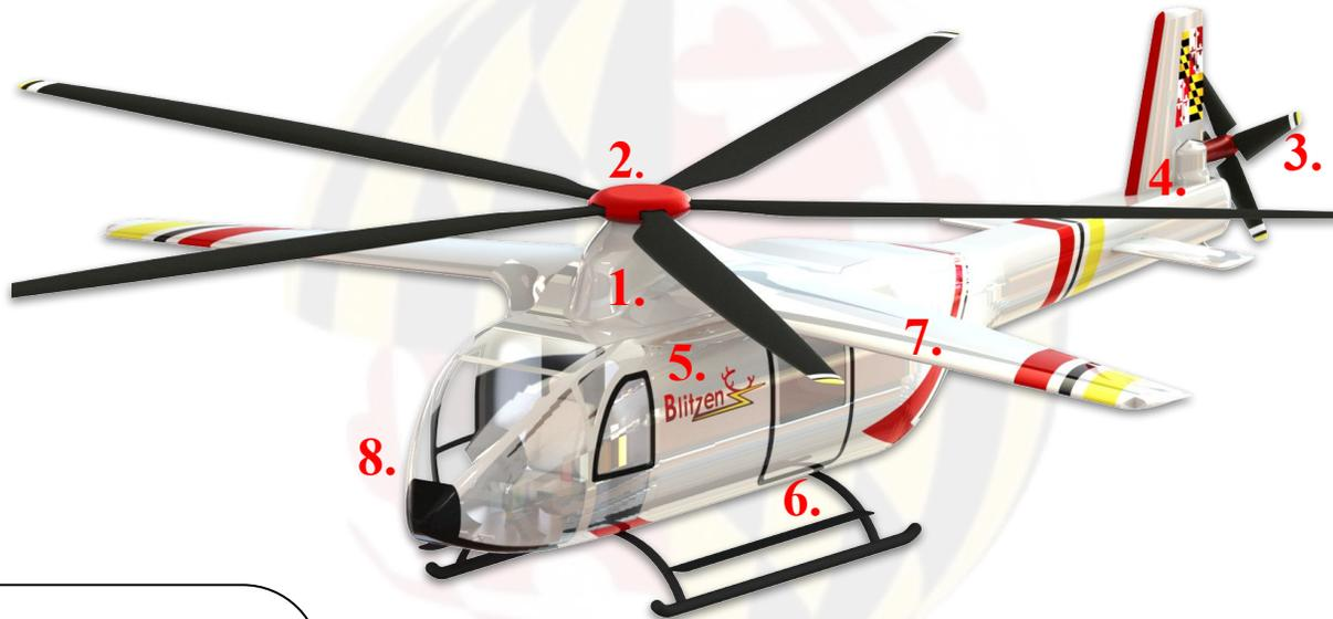
4. Swiveling Mechanism for anti-torque and forward thrust
