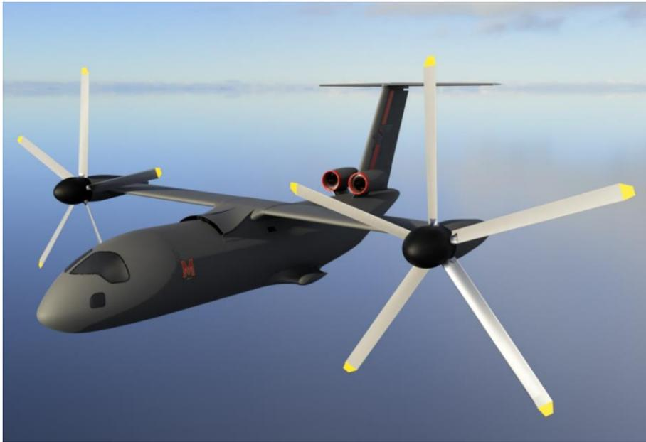
The AGRC-developed Arion is also endowed with unprecedented speed and embodies the immortal dream of VTOL – helicopter like hover and jet like cruise. Arion is a 48,000 lb **mixed power tiltrotor**, capable of delivering 5000 lb of cargo, or 20 fully
