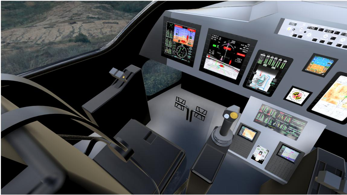
Figure 15.1: Cockpit controls including active side stick, split-power thrust control lever, and foot pedals.
