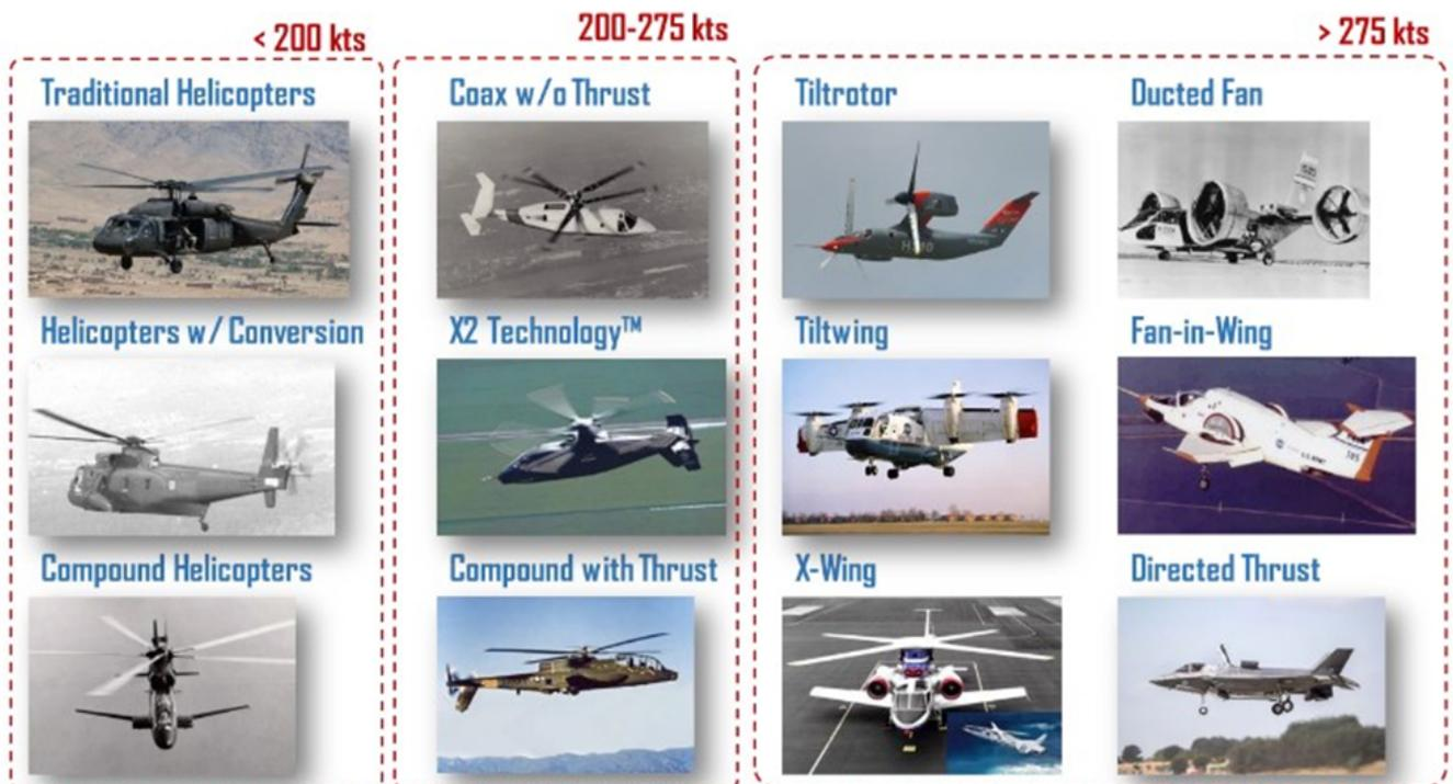
Figure 1.1: Tested VTOL Configurations Grouped by Top Speeds
