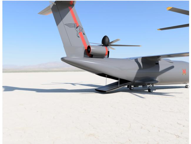
Figure 9.5: Rear cargo ramp open for loading cargo, vehicles, or personnel
