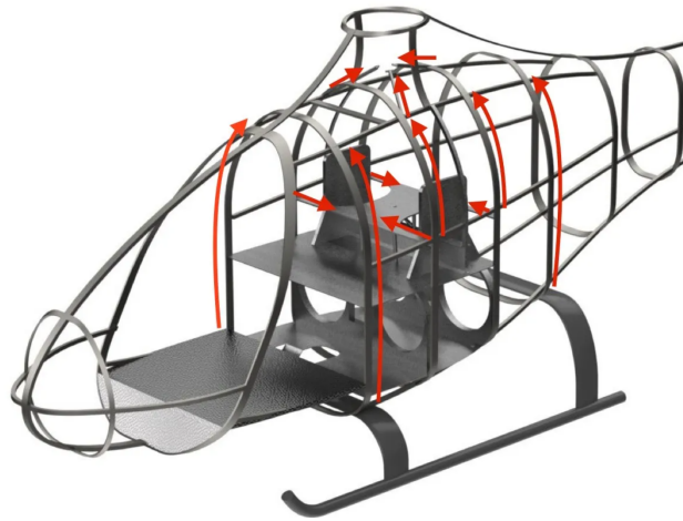
Figure 8.8: Fuselage Structure Load Paths
